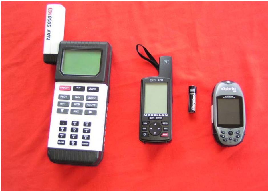
The original handheld; a 10 year oldie with a new Magellan & new Garmin with a AA battery for size comparison. The original uses 6 AAs every 2 hours, whereas new GPSs use 2 AAs every 12 hours.
